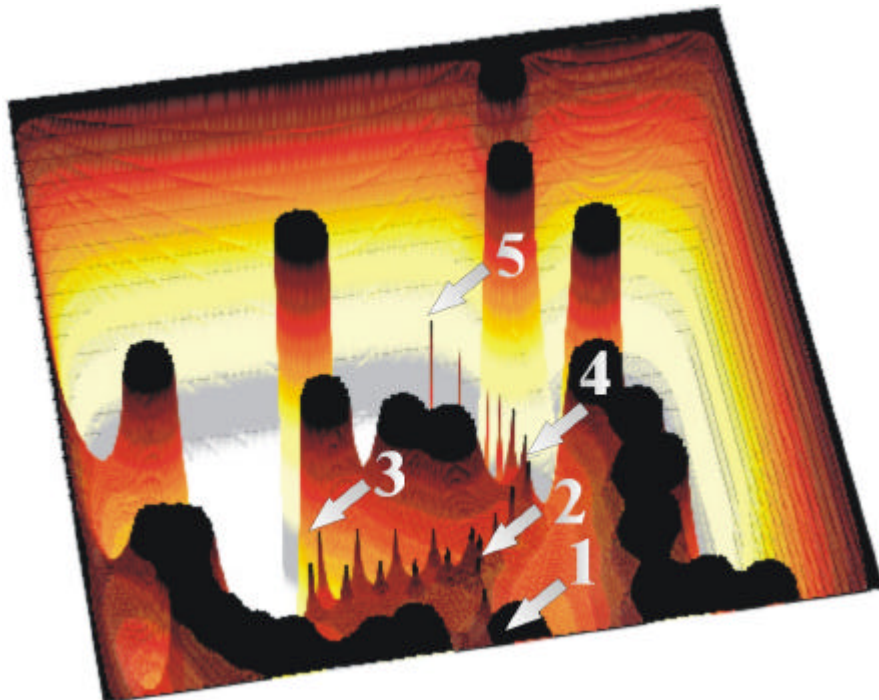
Figure 60: Robot making a large detour before reaching its target
